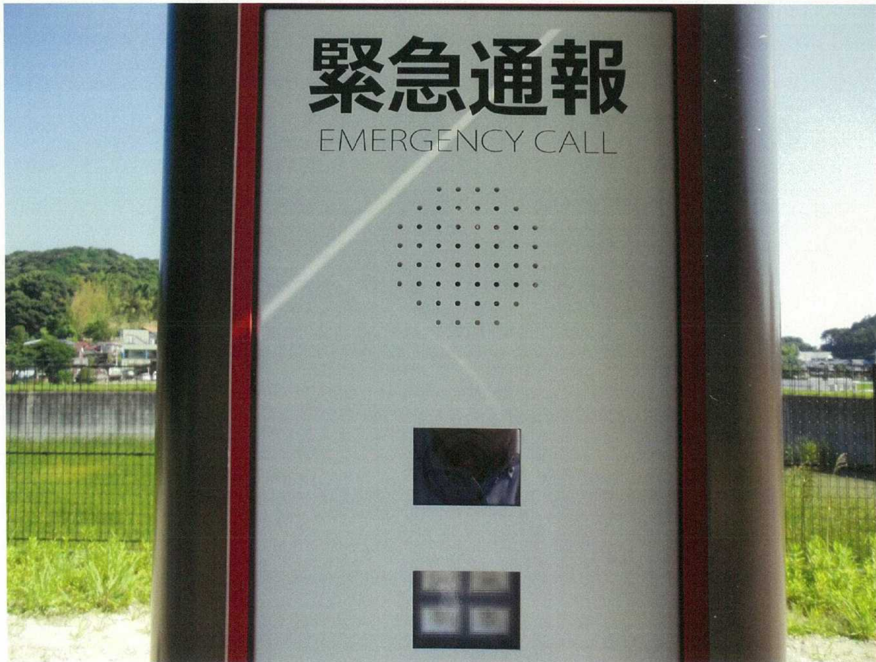
【Emergency call unit operating part upper part】
